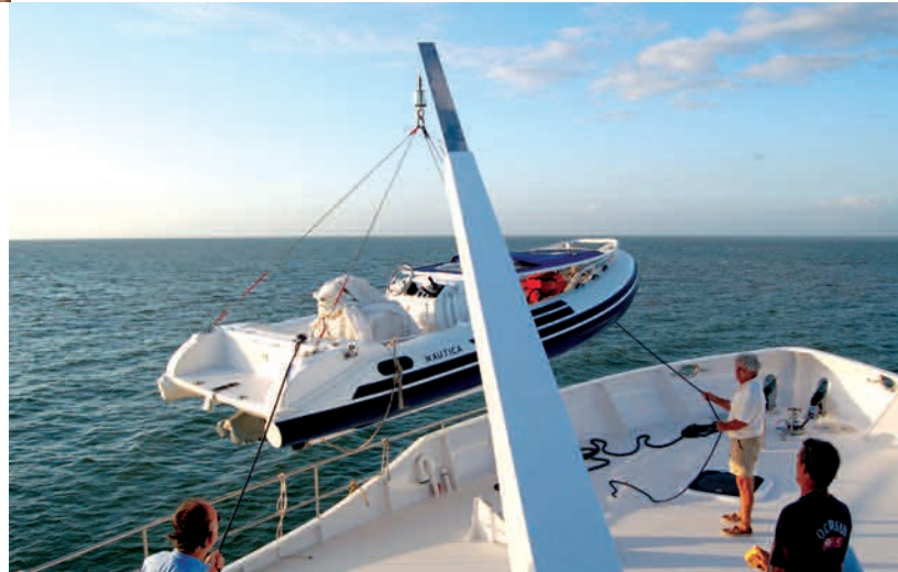
Top left: Maneuvering Aventura is simplified by the wing stations on the Portuguese bridge, equipped with shifters, thruster controls, and a joystick for steering. Above left: Owner Chuck Johnson, left, and builder Joe Johnson at the wing station. Above right: The 19-foot Nautica jet-drive RIB is easily launched on either side of the yacht by the 4,000-lb. Steelhead crane.
